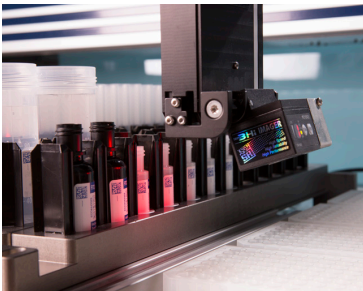
Scans IFA slide and reagent barcodes to ensure positive patient identification and assay integrity
