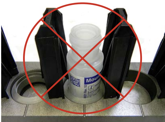
Figure 2-3: Incorrect Bottle Orientation
