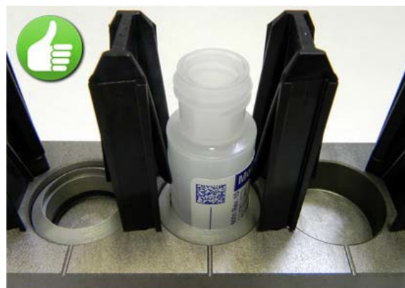
Figure 2-4: Correct Bottle Orientation
